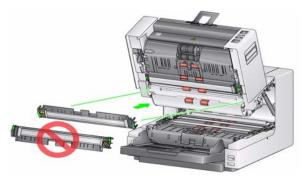
Loosen the upper flippable background accessory. Use a screwdriver to loosen all four screws.
