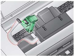
12. Open the ink cartridge package and remove the tab from the new ink cartridge.
