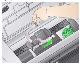
11. Push the connector on the printer cable firmly into the printer carrier.
