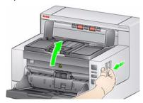
2. Loosen the screws on each end of the upper imaging guide and remove it from its position
