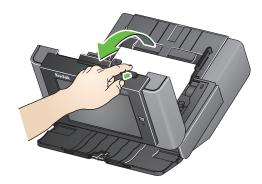
2. Remove any jammed document(s), close the Scan Station cover and resume scanning.
